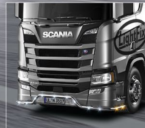
24741-6-P /-B - LightFix - FRONT-LINER "TARGA-MAX" Stainless steel LED-lightbar at the front with overrun protection polished or black powdercoated - Ø 60mm - prewired Full LED-set included
