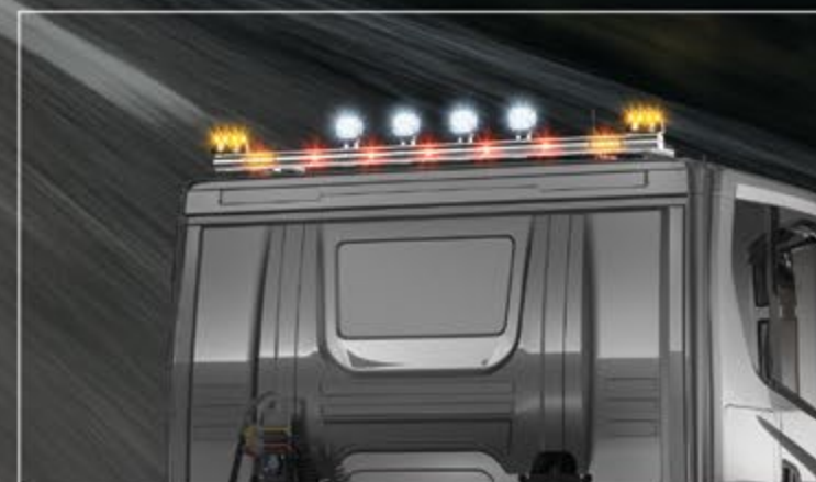
24716-1-P /-B - LightFix - REAR-LIGHT Lightbar for mounting a maximum of 6 work lamps and 2 beacons Stainless steel - polished or black powdercoated - Ø 70mm - prewired
