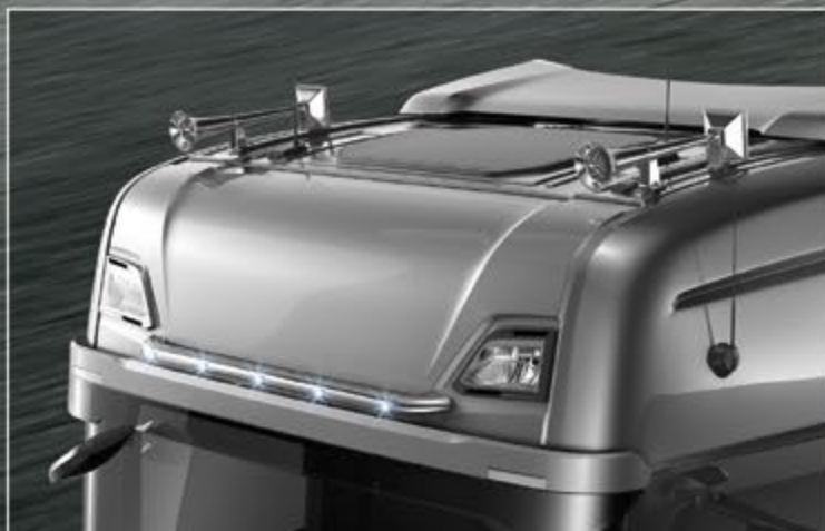
24705-11-P /-B - LightFix - SKY-LIGHT "VISOR" Lightbar including 5 integrated white LED stainless steel - polished or black powdercoated - Ø 70mm - prewired
