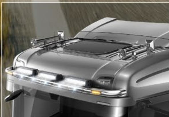
24705-P /-B - LightFix - SKY-LIGHT Lightbar for mounting a maximum of 4 / 6 spotlights stainless steel - polished or black powdercoated Ø 70mm - prewired
