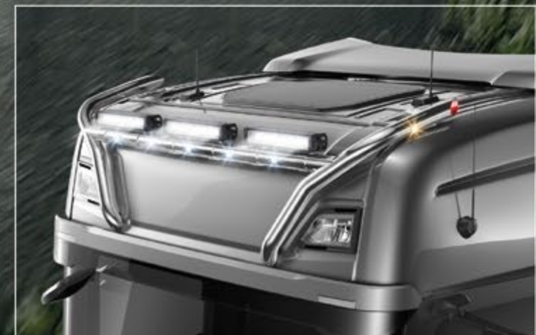
24705-8-P /-B - LightFix - SKY-LIGHT "WILDLIFE" Lightbar for mounting a maximum of 6 spotlights and 2 beacons stainless steel - polished or black powdercoated - Ø 70mm - prewired red LEDs in the tube ends
