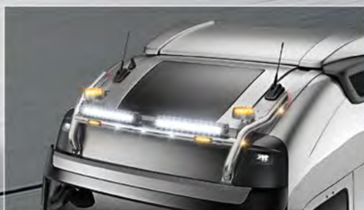
TLG23704-7-P / B - TLG23704-8-P / B - LightFix - SKY-LIGHT "WILDLIFE" Globetrotter (TLG23704-7-P / B) / Globetrotter XL/XXL (TLG23704-8-P / B) Lightbar for mounting a maximum of 6 spotlights and 2 beacons Stainless steel - polished or black powdercoated - Ø 70mm - prewired red LEDs in the tube ends included
