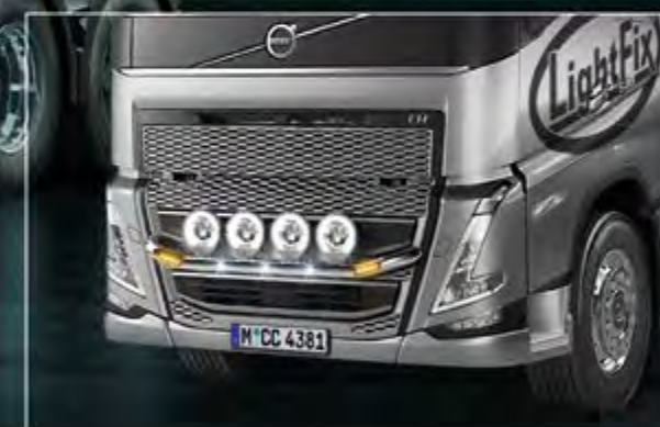
TLG23721-2-P /-B - LightFix - 4-LIGHT "MINI" Lightbar at the front for mounting a maximum of 4 spotlights stainless steel - polished or black powdercoated - Ø 70mm prewired
