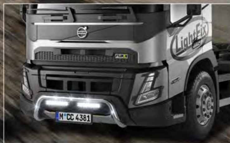
TLG23721-3-P - LightFix - 4-LIGHT Lightbar at the front for mounting a maximum of 4 spotlights stainless steel - polished - Ø 70mm - prewired
