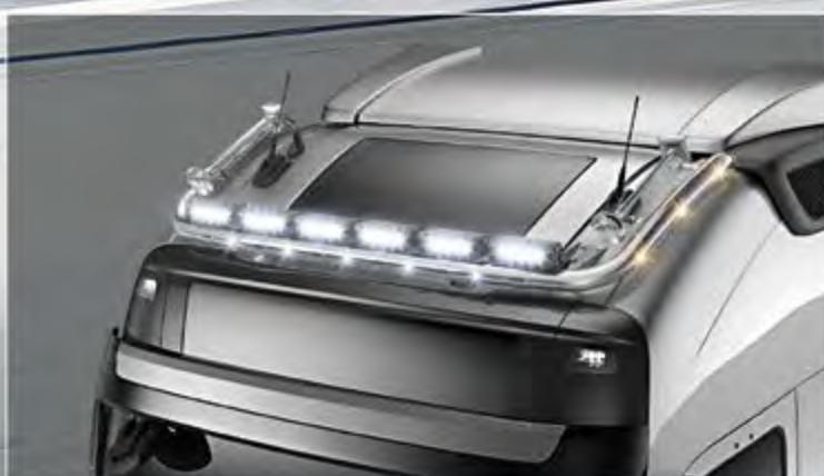
TLG23704-10-P / B - LightFix - SKY-LIGHT "BIG" Lightbar for mounting a maximum of 6 spotlights and 2 beacons stainless steel - polished or black powdercoated - Ø 70mm - prewired 6 amber LEDs on the side included
