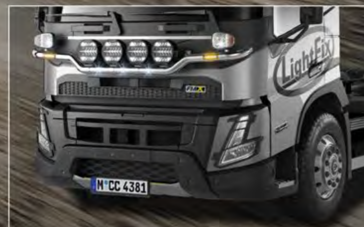
TLG23751-4-P - LightFix - PLOW-LIGHT Lightbar at the front for 2 main headlights and 4 spotlights Stainless steel - polished - Ø 70mm - prewired suitable for snow plows and municipal vehicles
