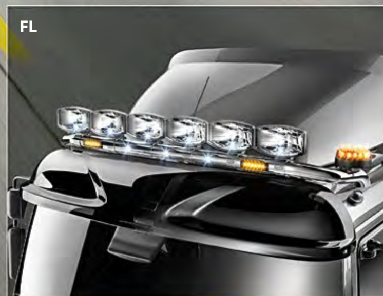
FL TLG23706-2-P - LightFix - SKY-LIGHT Lightbar for mounting a maximum of 6 spotlights and 2 beacons Stainless steel - polished - Ø 70mm - prewired
