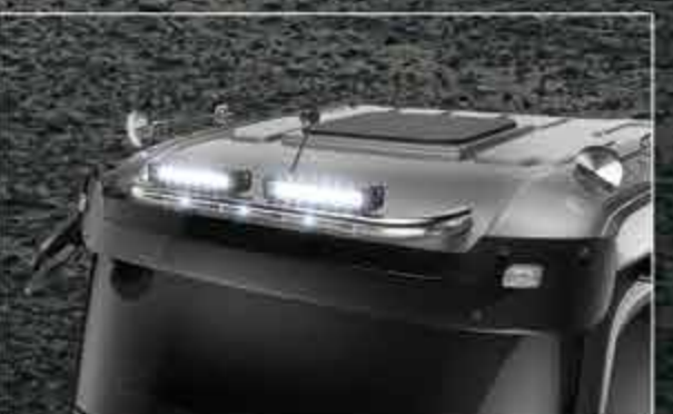
25704-2-P - LightFix - SKY-LIGHT "MINI" Classic Space Lightbar for maximum 4 spotlights and beacons stainless steel - polished or black powdercoated Ø 70mm - prewired
