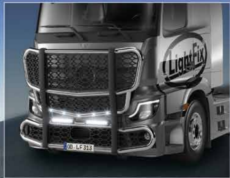
25761-2-P /-B - LightFix - FRONT-PROTECT "BIG NORDIC" Actros 2300 mm Stainless steel front protection bar incl. black net made of ABS polished or black powdercoated - Ø 70mm - prewired 29708-1-P /-B - LightFix - LAZER-BRIDGE for Lazer Triple-R 1000
