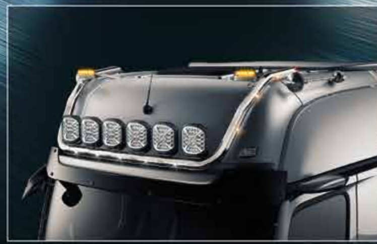
25707-3-P /-B - 25707-4-P /-B - LightFix - SKY-LIGHT Big Space (25707-3-P /-B) / Giga Space (25707-4-P /-B) Lightbar for mounting a maximum of 6 spotlights and beacons stainless steel - polished or black powdercoated - Ø 70mm - prewired red LEDs in the tube ends
