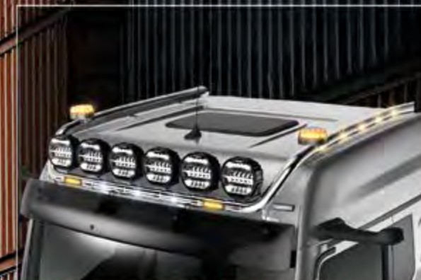
21703-5-P /-B - LightFix - SKY-LIGHT "WILDLIFE MAX" Lightbar for mounting a maximum of 6 spotlights and 2 beacons Full LED set and 4 light brackets included stainless steel - polished or black powdercoated Ø 70mm - prewired
