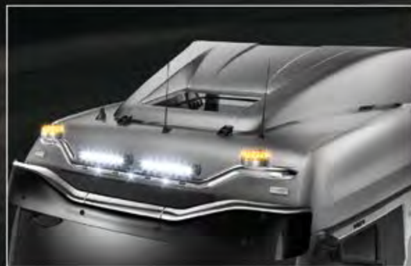
21702-8-P /-B - LightFix - SKY-LIGHT "WING" Lightbar for mounting a maximum of 4 spotlights and 2 beacons stainless steel - polished or black powdercoated Ø 70mm - prewired
