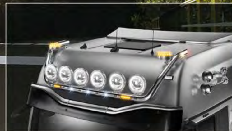
21706-4-P /-B - LightFix - SKY-LIGHT "WILDLIFE" Lightbar for mounting a maximum of 6 spotlights and 2 beacons stainless steel - polished or black powdercoated - Ø 70mm - prewired red LEDs in the tube ends
