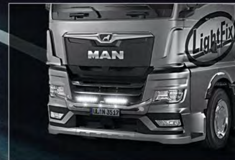
21720-6-P /-B - LightFix - 4-LIGHT "MINI" Lightbar at the front for mounting a maximum of 4 spotlights stainless steel - polished or black powdercoated - Ø 70mm - prewired
