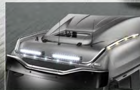
21702-7-P /-B - LightFix - SKY-LIGHT "H-MAX" Lightbar for mounting a maximum of 6 spotlights and 2 beacons stainless steel - polished or black powdercoated Ø 70mm - prewired incl. 8 amber LEDs on the side and red LEDs in the tube ends
