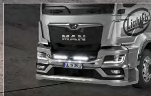
21720-6-P /-B - LightFix - 4-LIGHT "MINI" Lightbar at the front for mounting a maximum of 4 spotlights stainless steel - polished or black powdercoated Ø 70mm - prewired
