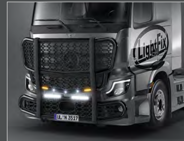
25761-2-B - LightFix - FRONT-PROTECT "BIG NORDIC" Actros Stream Space 2300 mm Kufanger i rustfritt stål inkl. sort nett i ABS sort pulverlakkert - Ø 70mm - montert kabel 29708-1-B - LightFix - LAZER-BRIDGE for Lazer Triple-R 1000
