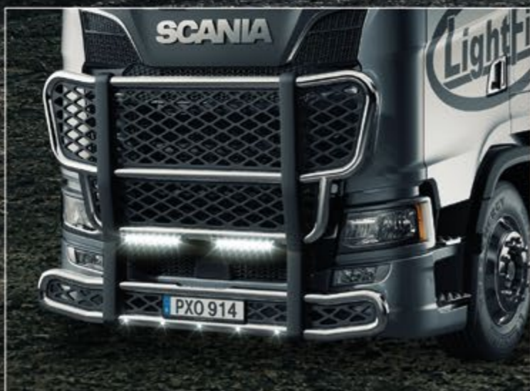
24760-2-P /-B - LightFix - FRONT-PROTECT "BIG NORDIC" Scania S / R - Bumper: Low Beam + Normal Beam Kufanger i rustfritt stål inkl. sort nett i ABS polert eller sort pulverlakkert - Ø 70mm - monteret kabel 29708-1-P /-B - LightFix - LAZER-BRIDGE for Lazer Triple-R 1000
