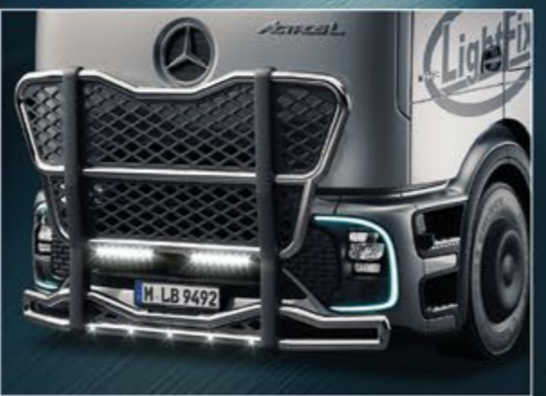
25760-4-P /-B - LightFix - FRONT-PROTECT "BIG NORDIC" Kufanger i rustfritt stål inkl. sort nett i ABS polert eller sort pulverlakkert - Ø 70mm - montert kabel 29708-1-P /-B - LightFix - LAZER-BRIDGE for Lazer Triple-R 1000
