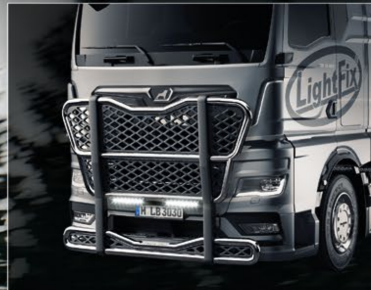
21760-4-P /-B - LightFix - FRONT-PROTECT "BIG NORDIC" Kufanger i rustfritt stål inkl. sort nett i ABS polert eller sort pulverlakkert - Ø 70mm - montert kabel 29708-1-P /-B - LightFix - LAZER-BRIDGE for Lazer Triple-R 1000
